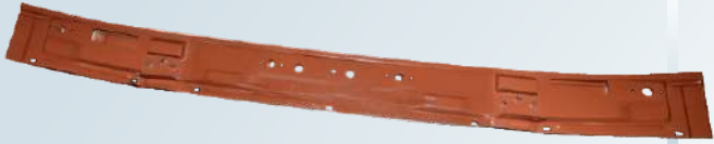
B 107 LPT WIPER PANNEL ASSEMBLY
